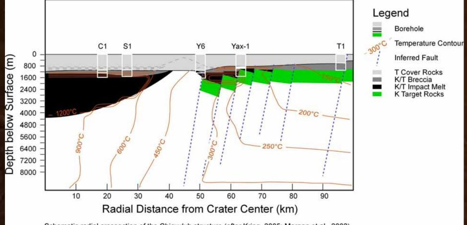
Schematic radial crossection of the Chicxulub structure (after Kring, 2005; Morgan et al., 2002), with a superimposed thermal model of Sudbury shortly after the formation of the crater (adapted from Ivanov and Deutsch, 1999, see also Abramov and Kring, 2004)
